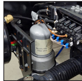
Chassis Air Dryer Relocation
