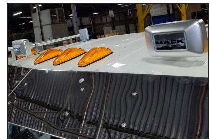
Horn: Air, Roof Mount Mack MD
