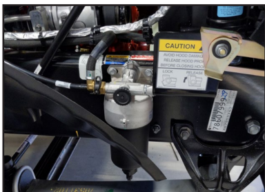
Chassis Fuel Filter Relocation
