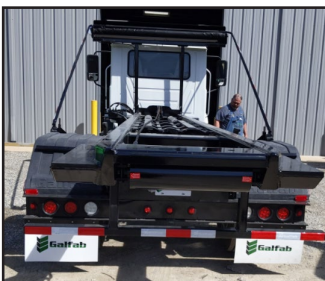
Chassis RollOff: 20ft, 20k, GALFAB
